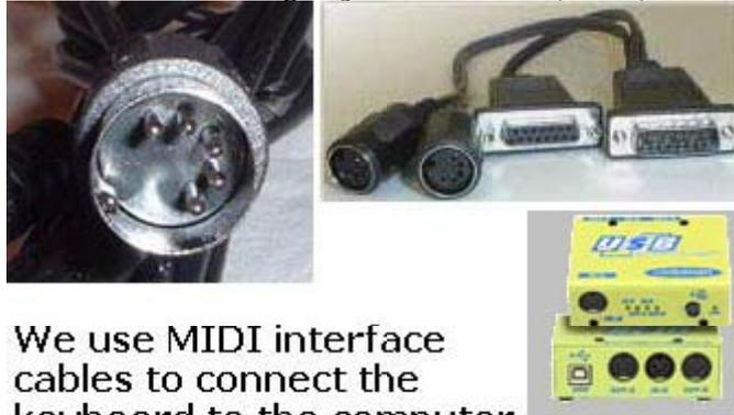
We use MIDI interface cables to connect the keyboard to the computer. USB to MIDI devices are also available.
