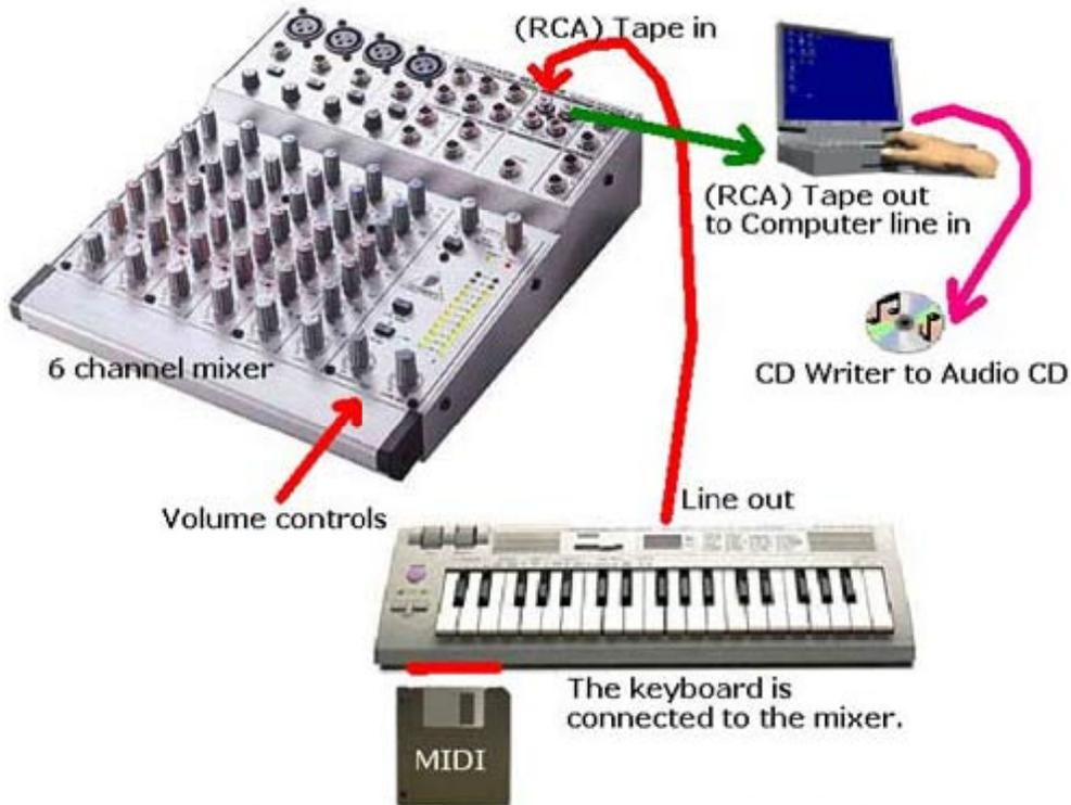
The keyboard is connected to the mixer.
